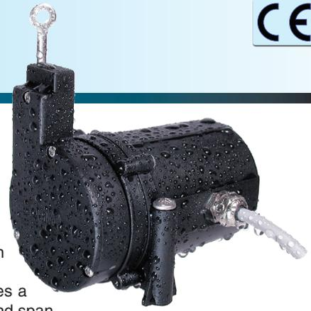
The JX-P420 series transducer is a loop powered device with a 4 to 20 mA current output that requires a two wire connection. The transducer, power supply, and current monitor are connected in series. Zero and span adjustment potentiometers are accessible by removing two sealing screws in the rear of the transducer housing. Zero and span allow for adjustment for a full 4 to 20 mA output at between 50% and 100% of maximum linear travel.
