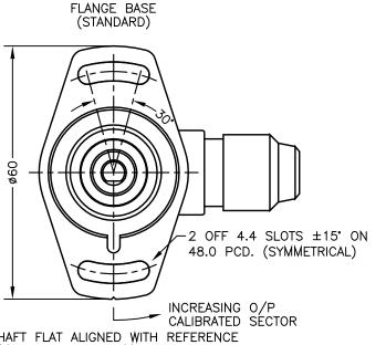
SHAFT FLAT ALIGNED WITH REFERENCE MARK IN BASE AT MID TRAVEL ±5°
