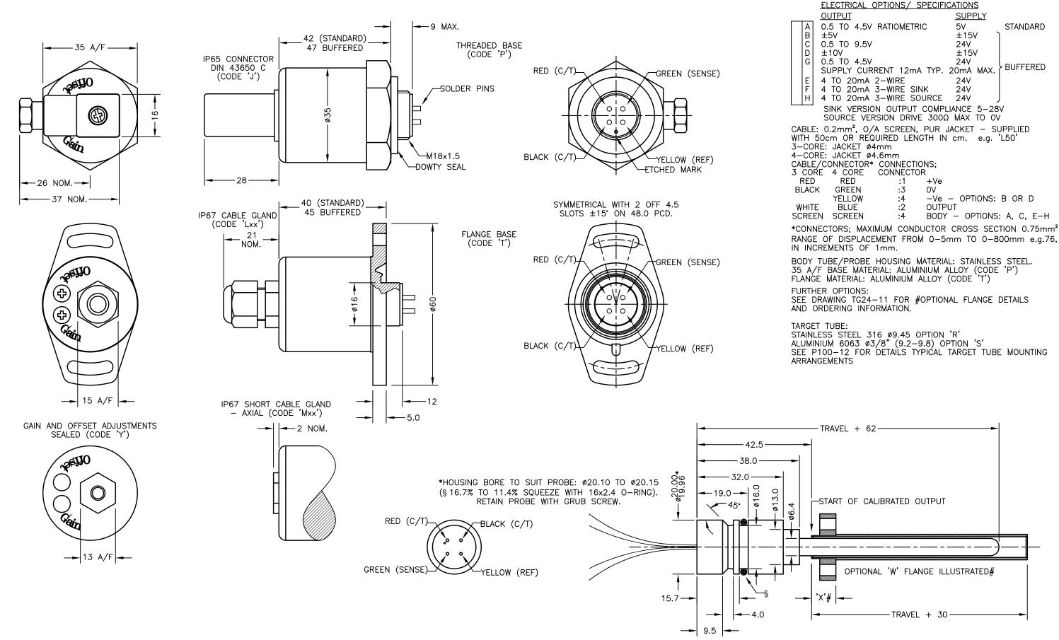
CONNECTIONS BETWEEN PROBE AND ELECTRONICS MODULE: FOUR WIRES; RED, BLACK, GREEN AND YELLOW, LENGTH: 300, CROSS SECTION: 0.25mm², WIRES POTTED IN PROBE HOUSING. INTERCONNECTIONS MUST BE PROTECTED FROM WATER INGRESS AND STRAIN RELIVED.
